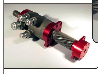
The drive adapter is machined from 4140 alloy steel and is screwed and bonded into the end of the pinion. As shown above, the slot accommodates the sensor's drive tab which is centered with an integral leaf spring.
