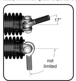
The clevis boot is extended onto a pressed-on machined aluminum lip, which prevents the boot from being stacked solid and thereby limiting rack travel.
