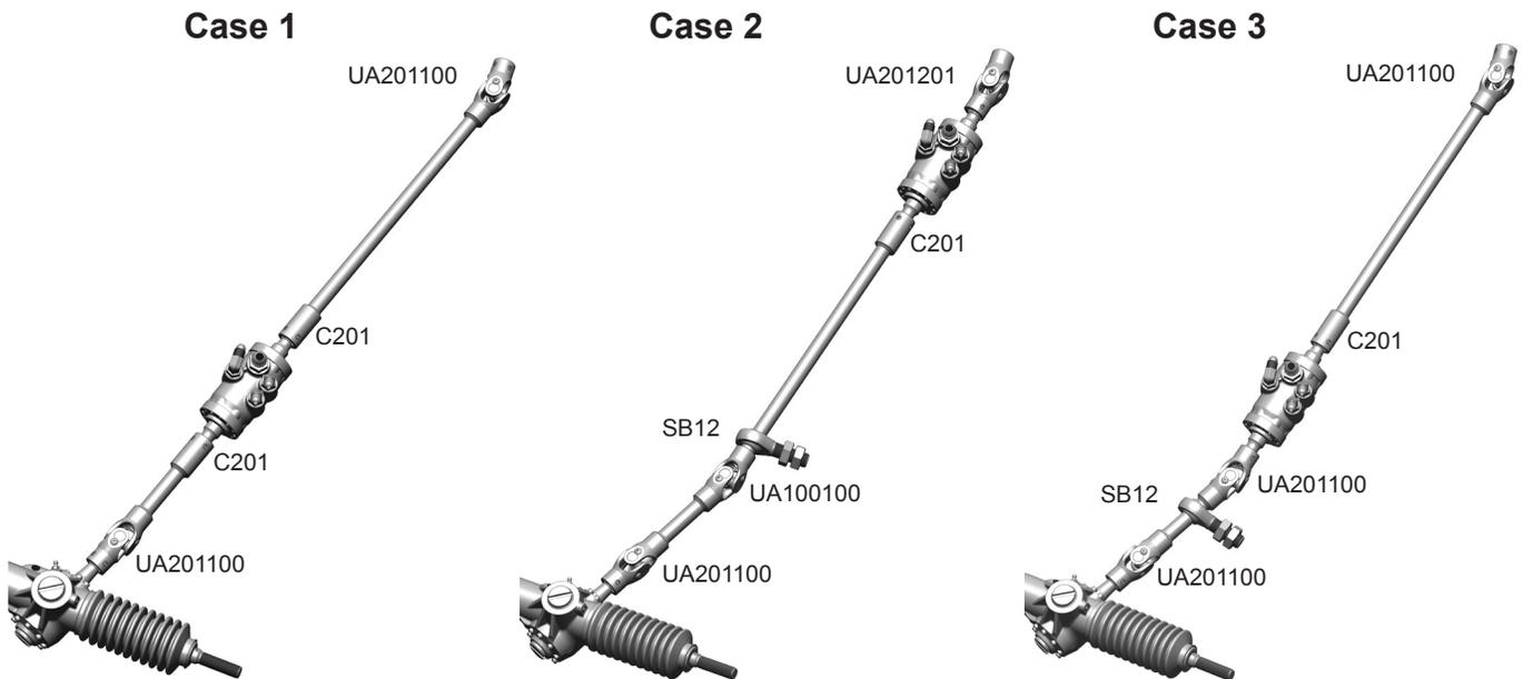
The simplest way to install a servo inline is to couple it into the intermediate shaft at any convenient point between the firewall bearing and the pinion. Since all the parts between the two u-joints are rigidly clamped together, the servo should be considered a solid part of the shaft.
