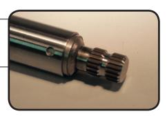
3. Weld through the 3 holes and around the end.
