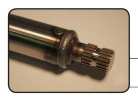
2. Insert the output spline, leaving about 1/8 inch for a circumferential fillet weld.
