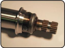
5. Weld the buttress ring in place. Note that this item prevents rearward movement of the steering column in a crash; treat it as you would a roll-cage joint. The recommended welding procedure is MIG, using ER80S-D2 wire with 75%Ar25%CO<sub>2</sub> shielding gas.
